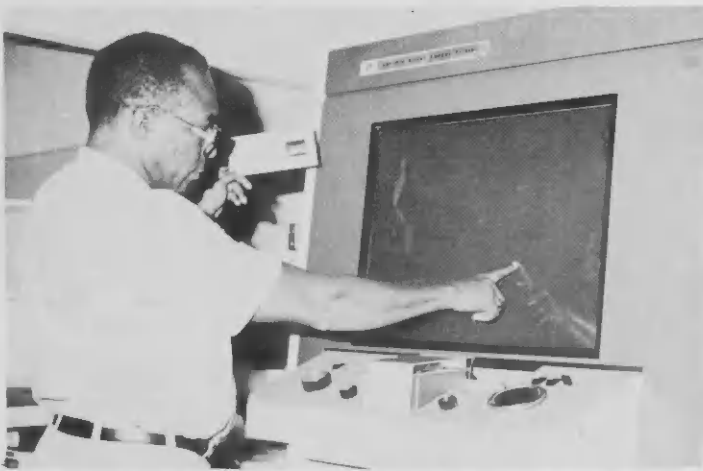
To have a view of the complete drawing, W. Wilson will insert one of those IBM aperture cards he is displaying in the aperture card machine in front of him.
